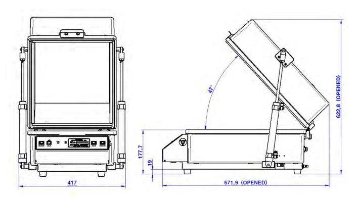
TC-5922BP Pneumatic Shield Box Data Sheet
