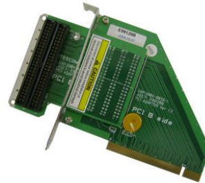
E99120B, PCI to 100pin adaptor, for the left side motherboard.
